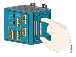
Step 3 Push up the upper module latches (at the top of the switch and the expansion module). See Figure B-4. Push down the lower module latches (at the bottom of the switch and the expansion module).
