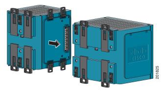
**Step 5** Push the upper module latches down and the lower latches up. See Figure 2-6.
