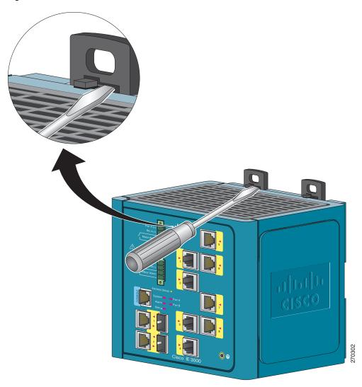
**Step 2** Push the DIN rail latches out. See Figure B-20.
