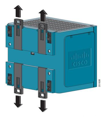
**Step 3** Position the rear panel of the switch directly in front of the DIN rail, making sure that the DIN rail fits in the space between the two latches.
