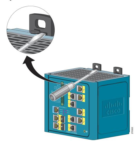
**Step 2** Push out on the DIN rail latches. See Figure 2-20.
