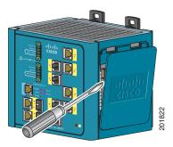
**Step 2** Remove the EMI protective cover from the interface connector on the switch. See Figure 2-2.
