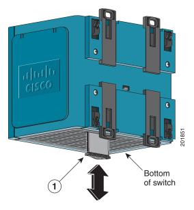
**Step 2** Install or remove the card, as desired:
