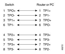
Figure C-8 Four Twisted-Pair Crossover Cable Schematics for 10/100/1000 Ports
