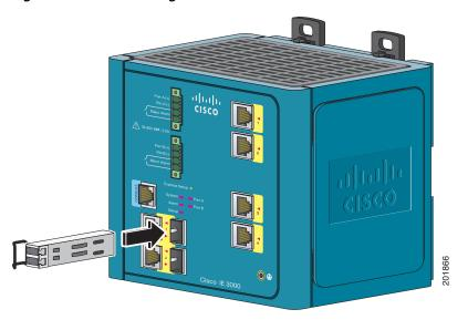
Figure 2-33 Installing an SFP Transceiver into an Module Port
