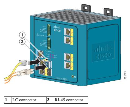
**Step 2** Connect the other end of the cable to the other device.
