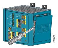
**Step 2** Remove the EMI protective cover from the interface connector on the switch. See Figure B-3.
