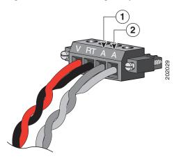
External device, relay wire A connection 1 **2** External device, relay wire A connection 2
