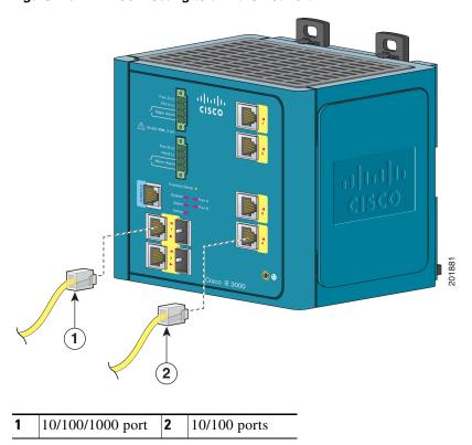
Figure B-31 Connecting to an Ethernet Port
