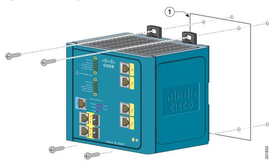
**Step 4** Place a number-10 screw that you provide through each DIN rail latch, and screw them into the wall.
