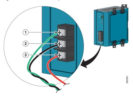
Figure 2-44 AC/DC Power Input Terminal Block Wire Connections to a DC Source
