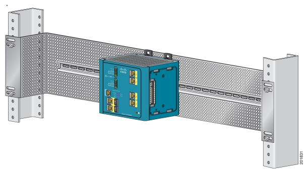
After the switch is mounted in the rack, connect the power and alarm wires, as described in the "Connecting Power and Alarm Circuits" section on page B-39.
