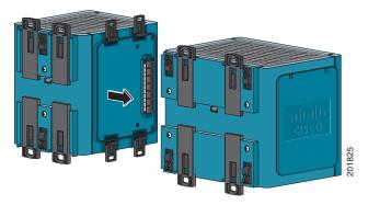
**Step 5** Push the upper module latches down and the lower latches up. See Figure B-6.
