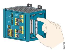
Push up the upper module latches (at the top of the switch and the expansion module). See Figure 2-4. Push down the lower module latches (at the bottom of the switch and the expansion module).
