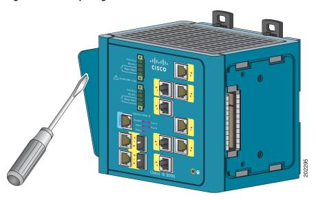
**Step 2** Push the upper modules latches (at the top of the switch and the power converter) up and the lower module latches (at the bottom of the switch and the power converter) down. See Figure 2-39.
