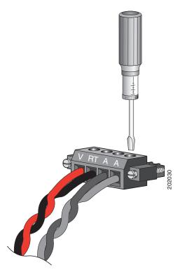
**Step 5** Repeat Step 1 through Step 4 to insert the input and output wires of an additional external alarm device into the second power and relay connector.
