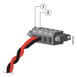
1 Power source positive connection 2 Power source return connection
