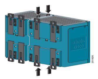
**Step 6** If you are going to install a second expansion module to the switch expansion module combination, follow Step 1 through Step 5.
