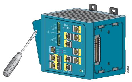
**Step 2** Push the upper modules latches (at the top of the switch and the power converter) up and the lower module latches (at the bottom of the switch and the power converter) down. See Figure B-39.
