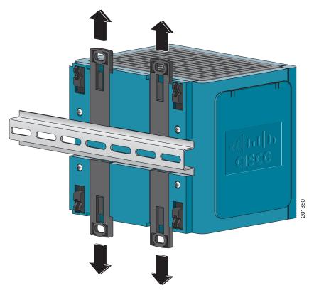
Figure 2-27 Removing the Switch from the DIN Rail
