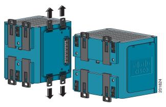
Step 4 Align the connectors on the switch and the module, and slide the switch and the module together to make the connection. See Figure 2-5.
