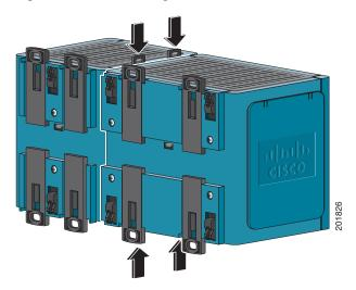
Step 6 If you are going to install a second expansion module to the switch expansion module combination, follow Step 1 to Step 5
