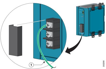
Figure 2-42 AC/DC Power Input Terminal Block
