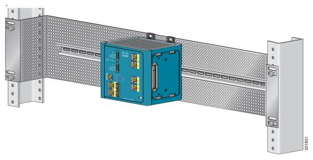
After the switch is mounted in the rack, connect the power and alarm wires, as described in the "Connecting Power and Alarm Circuits" section on page 2-36.
